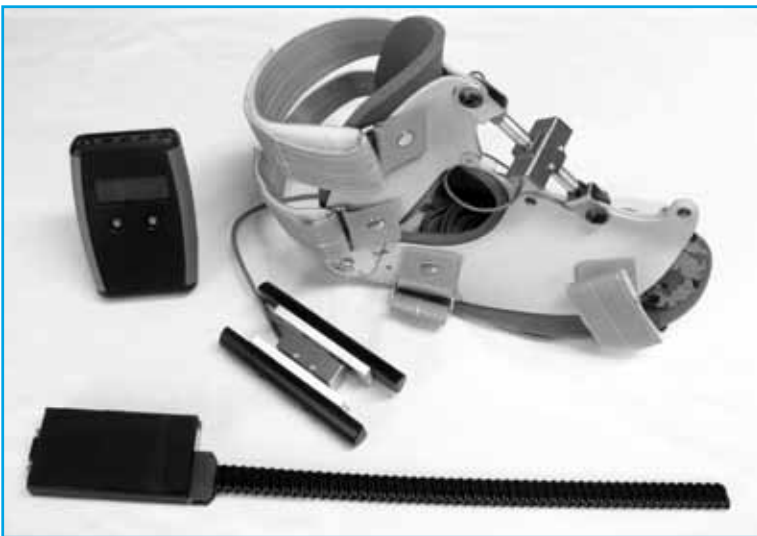
Prototype devices for measuring strength and mobility, from the “Doctor is in the House” kit
